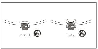
Step 4 Finally, adjust the link and drain lever position to ensure the drain can be fully opened and closed. Run water into the washbasin to ensure drain is functioning well and inspect all the connections for leak.
