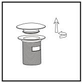
Step 1 Remove flange and rubber gasket from drain body. Flange can be unthreading in anti-clockwise direction.
