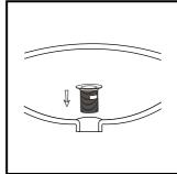
Step 2 Place rubber gasket in place over the drain From underneath of basin, reattach the hole in basin, follow by inserting the flange flange to drain body by threading it in into the drain hole.
