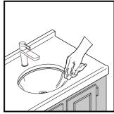
Carefully remove excess silicone sealant immediately. Install the faucet and drain directions, each clip is rotated over the rim. according to respective installation guides.
