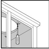
Step 2 Make sure the underside of countertop and rim of basin are dry and clean from dirt. Loosely install the mounting clip.
