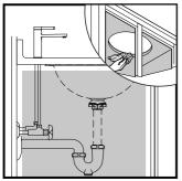
Step 1 Place the washbasin on the cut-out countertop to verify proper fit and cabinet clearance.
