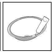
Step 3 Apply silicone sealant to the ground rim of basin (Do not use epoxy resin or rigid adhesive as this may cause the basin to crack).
