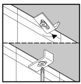
Step 4 Hold the basin in place under the opening of countertop, ensure basin is level in all Secure the basin in position by evenly tighten the clips.
